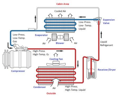
Automobile A/C Schematic Arrangement
