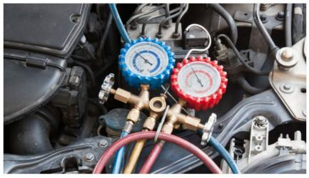
A/C Manifold Pressure Gauges
