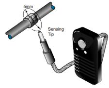
When set at its highest sensitivity, it can detect a leak of 1/10 ounce per year.
