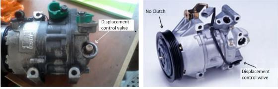
Internally Controlled Variable Displacement Compressor
