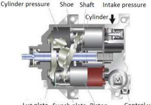
Lug plate Swash plate Piston Control valve
