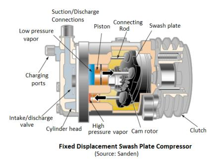
For compressors with fixed inclination swash plate angle, piston stroke is also fixed and the cooling capacity of the compressors changes only with the engine operating speed. The cooling load for the compartment can only be controlled by ON-OFF control of compressor clutch attachment to the engine shaft.
