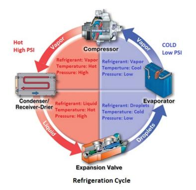
In the figure above, note that the high-pressure side of the system extends from the outlet of the compressor to the metering device (expansion valve). The low-pressure side extends from the expansion valve back to the inlet of the compressor.
