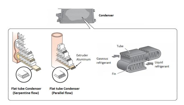
Some systems use multiple-path condensers with two or three shorter serpentine sections connected in parallel. This maximizes the time the refrigerant stays in the condenser for increased heat transfer.
