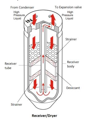
The outlet of the receiver/dryer connects to a siphon tube that goes to the bottom of the container. This acts as a liquid/vapor separator and ensures only liquid refrigerant is supplied to the
