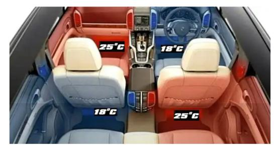
A car equipped in 4-zone system would obviously be expensive because of the presence of additional sensors and a complex electronic control unit.
