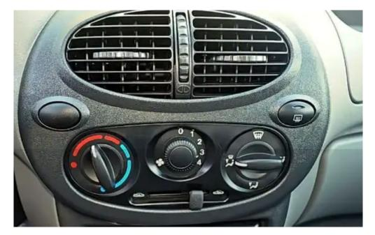
The driver sets the temperature and the speed to control the amount of cold air.
